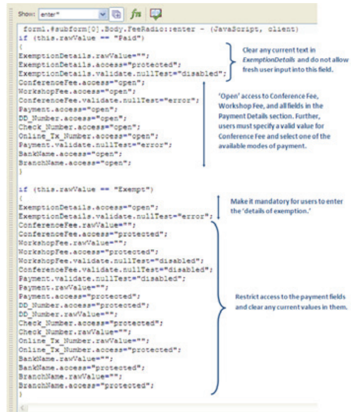
Figure 4. Implementing conditional fields using basic scripting
